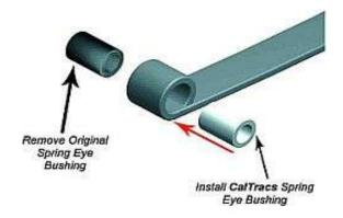
Now you are ready to install the CalTracs and reinstall the rear springs into the car.
