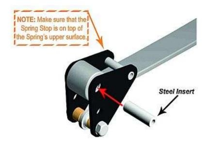
With each spring assembly ready to go in, position the Front Pivot assembly to the front spring eye. (Assure that the Spring Stop is located on the upper surface of the spring). Install the Steel Insert through the pivot and front spring eye bushing. Now, reinstall the spring using the original hardware. Repeat the process for the other side.
