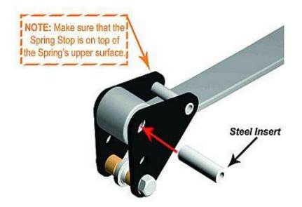
With each spring assembly ready to go in, position the Front Pivot assembly to the front spring eye. (Assure that the Spring Stop is located on the upper surface of the spring). Install the Steel Insert through the pivot and front spring eye bushing. Now, reinstall the spring using the original hardware. Repeat the process for the other side.
