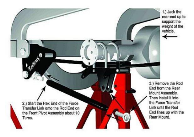
With CalTracs installed, reinstall the rear tires and lower the car to the ground. For an initial setting, have the driver in the car, (or a similar amount of weight). Turn the Force Transfer Link until the Spring Stop Bolt just contacts the upper surface of the spring, then turn the Force Transfer Link 1/2 Turn evenly side to side to establish pre-load. Tighten the Force Transfer Link lock nut. **All done!**
