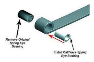
Now you are ready to install the CalTracs and reinstall the rear springs into the car.
