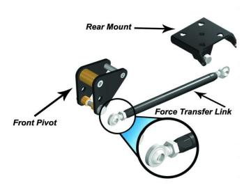
forward). This is where the system emulates a Four Link System. The pinion angle is also maintained.
